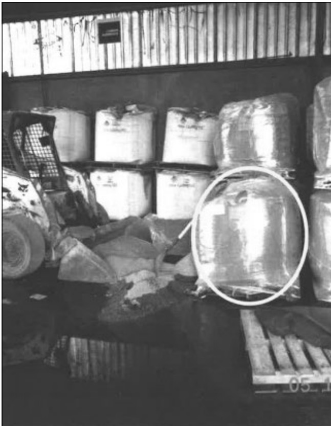
The lower tiered super-sack of tap hole sand (white circle) where the hole was located.
