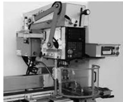
**4. Self-adjusting guards** in which the size of the opening in the barrier adjusts to accommodate the stock, e.g., enlarges to allow larger stock to enter.
