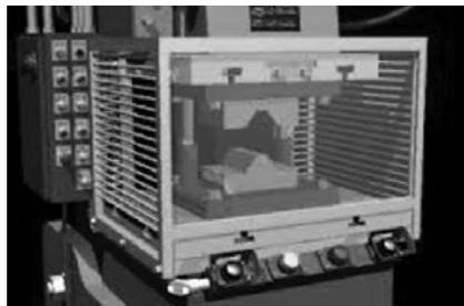
**(Note:** The machine guard in our "Spot the OSHA Violation" quiz above is also a fixed guard; but its openings are too wide to keep a worker from reaching into the guard and making contact with the point of operation.)
